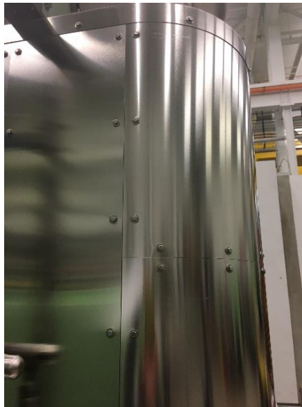
Magnetic shields using rivet assembly
