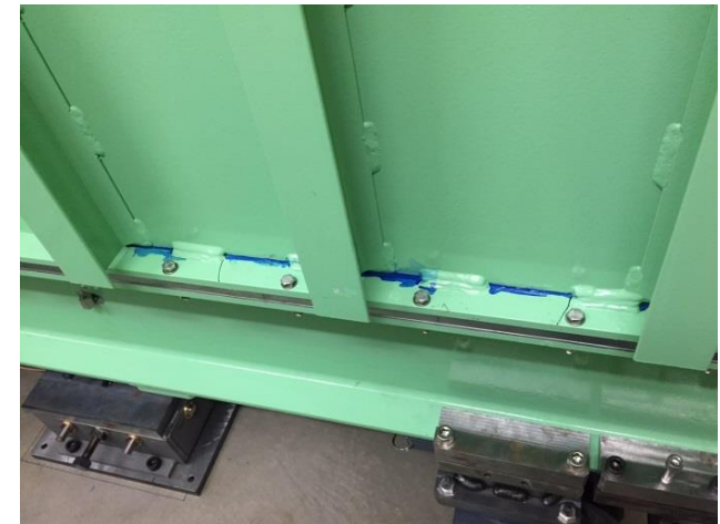
\beta=0.53 cryomodule vacuum vessel welding defect
