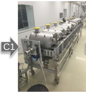
Completed cold mass assembly in clean room
