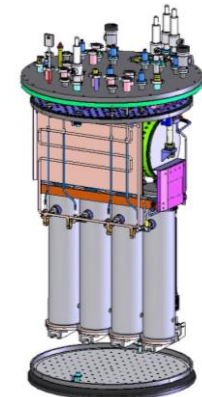
INFN Legnaro (QWR, top down) operating –common vacuum
