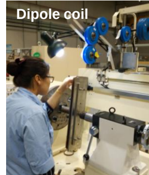
Winding of the solenoid at the vendor
