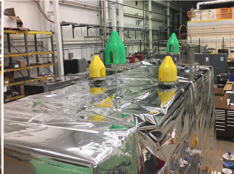
Protective covers for vacuum cover penetrations during installation
